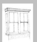
Even where 'glazing bars' are inserted into the glass cavity, the flatness of the window remains a problem. Replacement windows often require subtle alterations to the window opening, with loss of proportion and scale.
